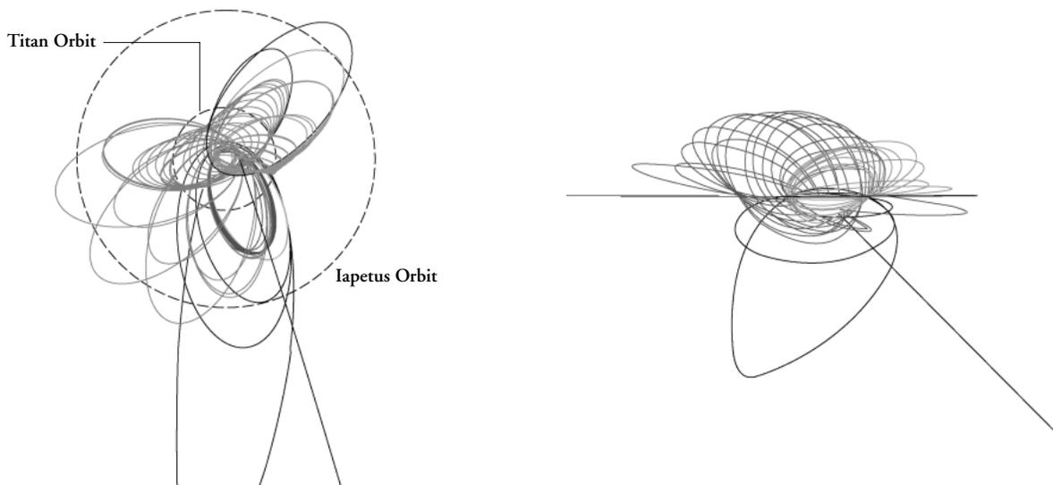
Figure 2. The Cassini orbiter’s “tour” of Saturn’s system is traced with orbital tracks around Saturn. The left diagram is a “petal plot” with the view looking down on Saturn’s north pole.
